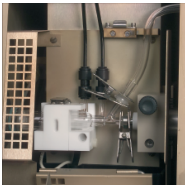
Figure 2: XSeries II dual mode sample introduction for GC-ICP-MS
