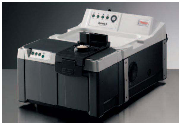
Figure 2: Antaris FT-NIR Solid Sampling system with Sample Cup Spinner
