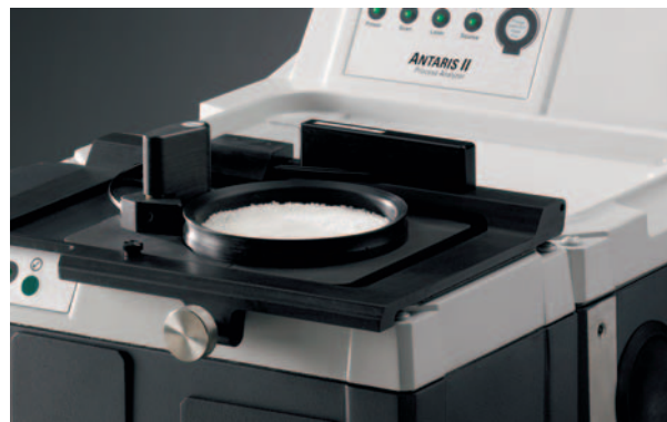
Figure 1: Sample Cup Spinner for the Thermo Scientific Antaris™ FT-NIR analyzer
