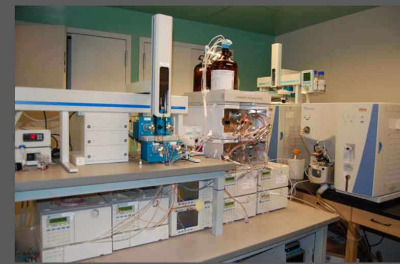
TFC MS/MS system: Thermo Aria TLX-2 – Turbulent Flow Chromatography System and Thermo TSQ Vantage
