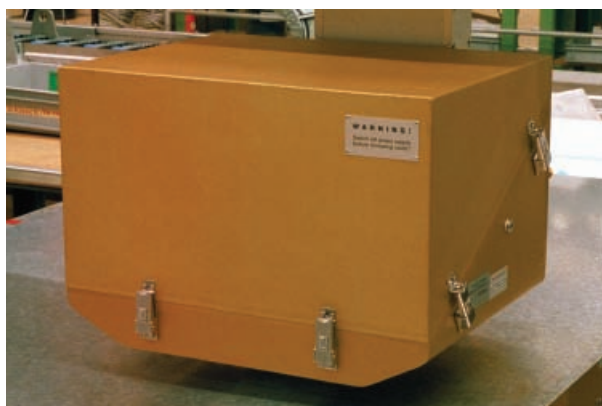
X-ray Fluorescence Measuring Head for One Side of the Coated Strip
