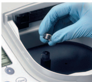
Light Sealing Lid accessory used with the nanoCell
