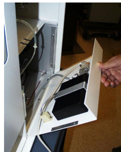
Installing modem located on replacement panel.
