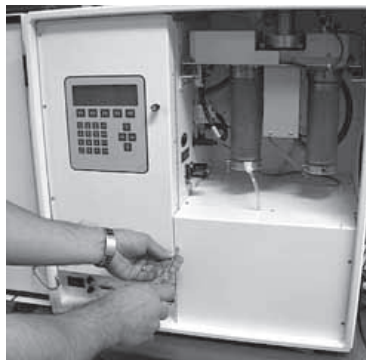
Removing pump compartment panel for installation of modem kit.
