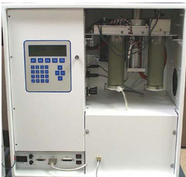
Front view of Partisol-Plus Sampler with modem kit installed.
