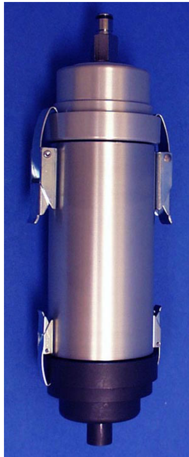
ChemComb cartridge with 10 l/min PTFE-coated PM-2.5 inlet on the bottom, and modular sample flow exit at the top.
