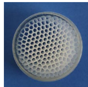
View looking through a honeycomb denuder.
