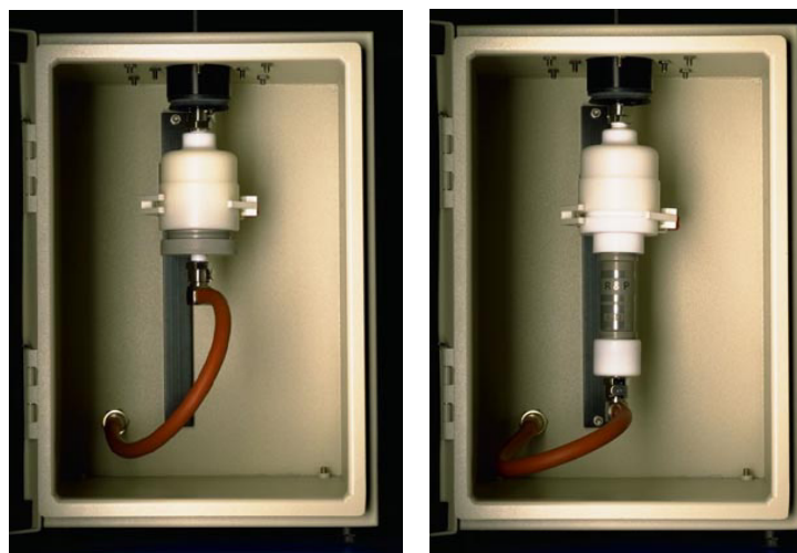
Four-Stage Filter Pack (left) and PUF Sampling System installed in Partisol satellite units.
