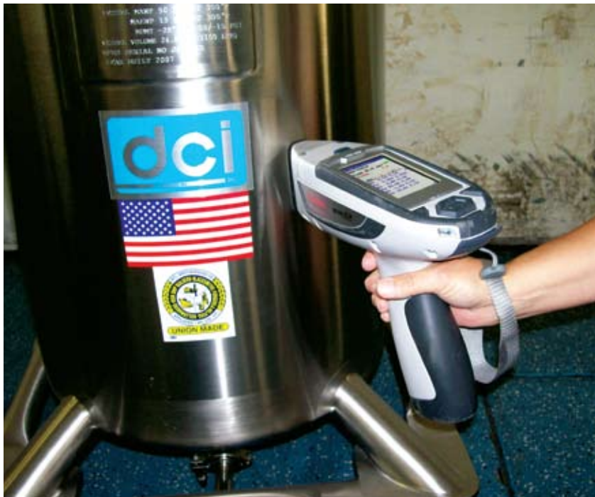
A final quality check of a vessel liner for use in the biopharmaceutical industry ensures that there will be no compatibility issues. Source: Thermo Fisher Scientific
