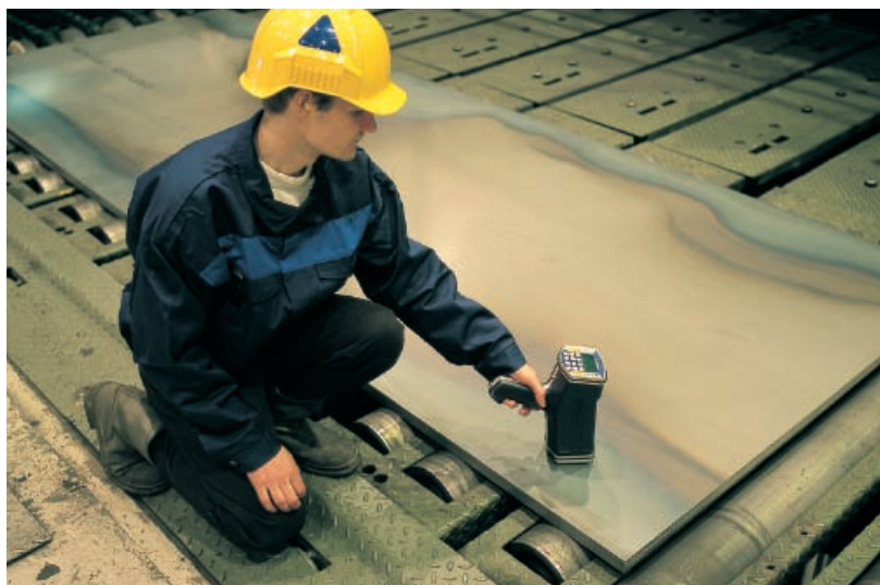
Oil Film Measurement with the SC 4000
