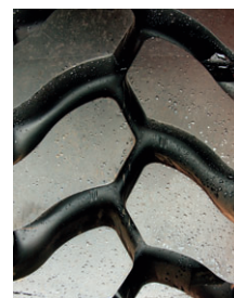
Figure 1: Carbon black rubbers, such as this tire, represent a challenging sample for infrared analysis
