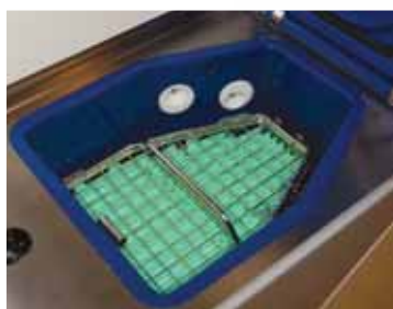
Secondary chamber capable of processing 60 cassettes
