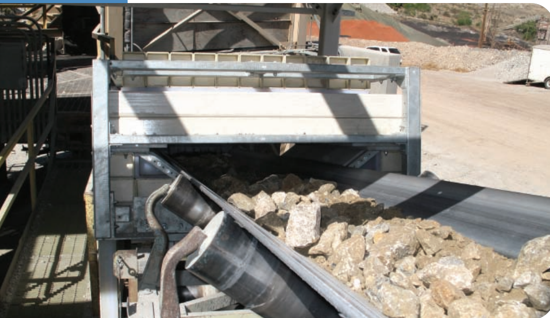
CB Omni cross-belt online elemental analyzer
