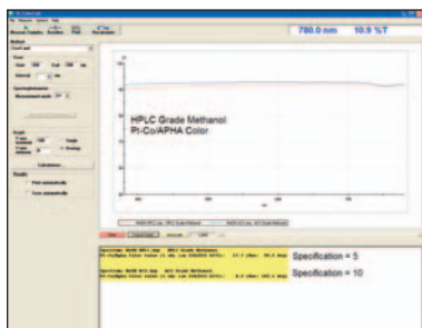
Automatic APHA color measurements are available with the VISION/ite ColorCalc application software.
