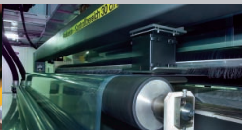
Thermo Scientific Mark III scanner on the stretch film line C05
