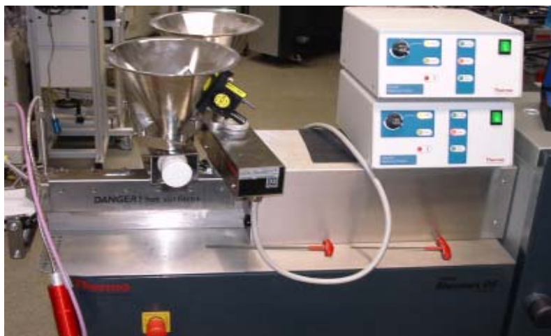
Fig. 2: Separate Feed of wax and powder.
