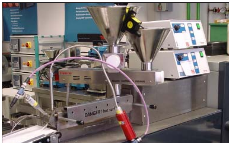
Fig. 1: Instrument setup, RD16, PTW16/25, split feed with two metering feeders, die plate and conveyor belt.
