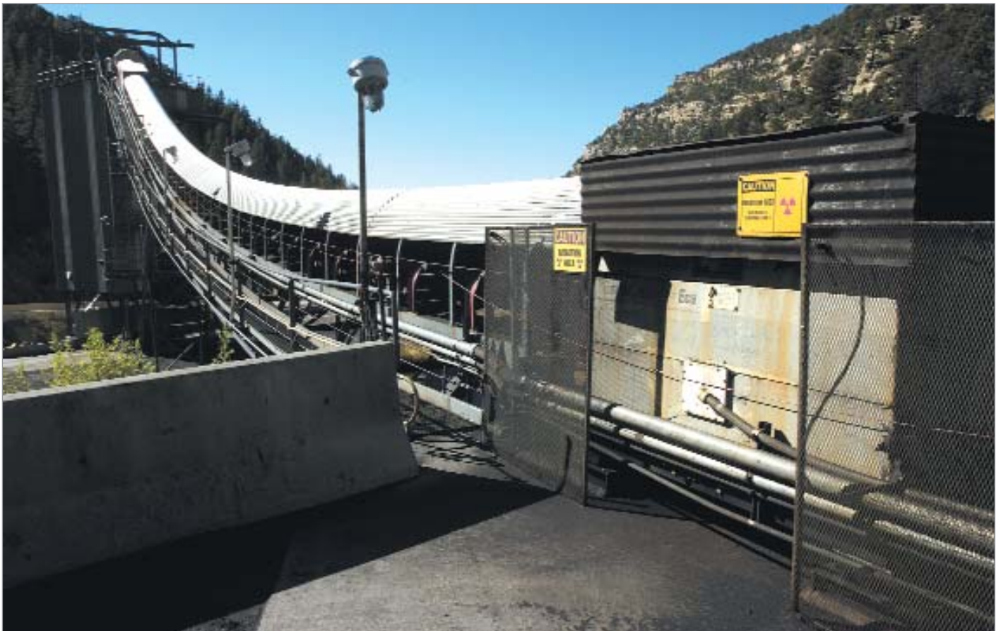
Figure 4. The Gamma-Metrics ECA coal analyser fits around existing conveyor and provides minute-by-minute analysis of sulphur and ash.
