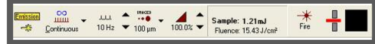
FIGURE 4. Laser parameters used with the New Wave UP213. Sample was moved at a rate of 5 µm/s over a line of 500 µm.
