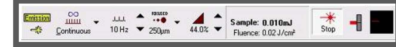
FIGURE 7. Pre-ablation parameters and fluence with the New Wave UP213. Sample was moved at a rate of 200 µm/s over a 5 mm square.
