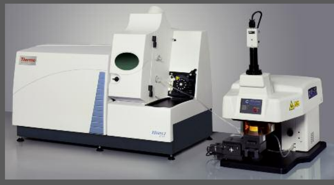
FIGURE 1. Thermo Scientific XSERIES 2 ICP-MS and New Wave UP213 SA (switchable aperture) Laser Ablation system used in these analyses.
