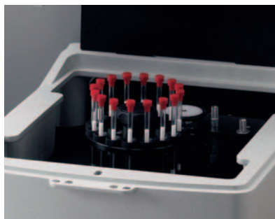
The DXR SmartRaman spectrometer with the Carousel Autosampler Sampling accessory
