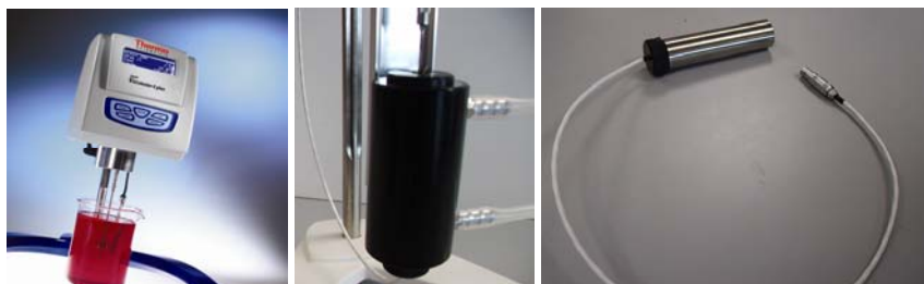
Fig. 1: HAAKE Viscotester 7 plus with 600 ml beaker and temperature sensor, which belongs to the standard contents of delivery (left), mounted adapter with temperature vessel and liquid temperature control (middle), sample vessel with integrated temperature sensor for HAAKE Viscotester 7 plus (right)
