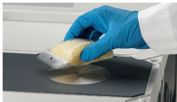
Figure 2: Typical sample scanned on the Integrating Sphere of the Antaris II FT-NIR system. Samples were easily scanned through the plastic bag in about 15 seconds.
