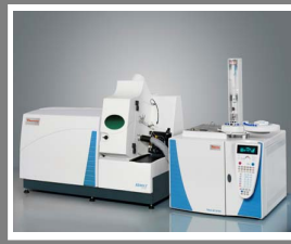
FIGURE 3. Thermo Scientific Trace GC Ultra coupled to the XSERIES 2 ICP-Q-MS
