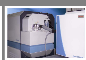
FIGURE 9. Trace GC Ultra coupled to the Thermo Scientific ELEMENT 2 ICP-SF-MS
