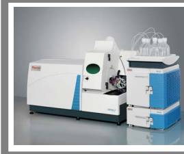
FIGURE 2. Thermo Scientific Accela U-HPLC coupled to the Thermo Scientific XSERIES 2 ICP-Q-MS
