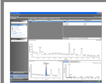
FIGURE 4a. Review of Survey Screening results showing the peaks found and the mass spectrum of the highlighted peak.
